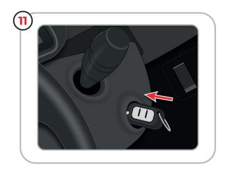
Insert key in ignition barrel, turn on fully then off again fully, ensure the dash is not illuminated and you **must** leave the key in the ignition to disable the steering lock.
