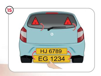
You **must** fit the number plate of tow vehicle to rear of towed vehicle, you **must** fit obligatory rear reflective triangles.
