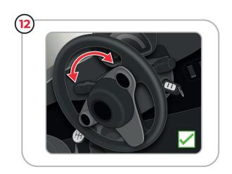
Check the steering lock is disabled and the steering wheel free to move by turning left and right half a turn.
