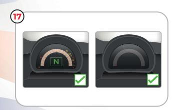
The dash display/screen **must** be fully asleep e.g., no display showing before towing. (Some models may take 2 mins to go to sleep), if practicable close the car and lock it.
