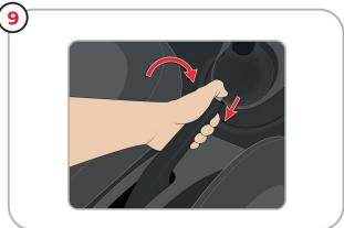
ONLY when the tow ball is connected and safe to do so release parking brake (cover the foot brake in case the vehicle moves – if vehicle static proceed).
